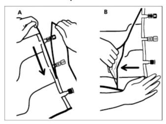
• To remove overpouch, hold the bag horizontally and tear from the notch close to the ports along the upper edge (A).
