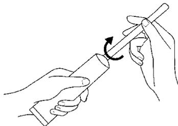
3. Screw the applicator to the tube, and fill the applicator by squeezing the bottom of the tube until the plunger is fully extended.
