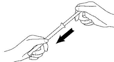
After each use, wash the applicator thoroughly. It can be taken apart by firmly pushing the head of the plunger up inside the cylinder. Withdraw the plunger from the cylinder. Wash the parts in warm water, with a mild detergent, and rinse thoroughly. Reassemble by pushing the plunger into the cylinder.
